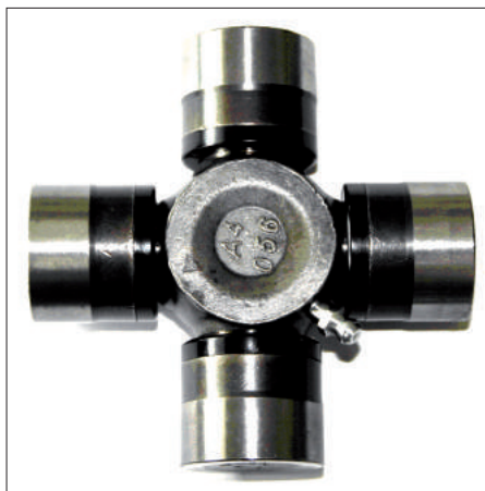
Variante / Type 7 7 = LS Lateralschmierung Lateral Grease Nipple
